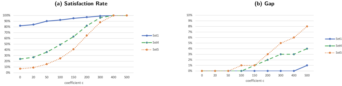
Figure 2: Effect of coefficient c on the quality of the solutions of eNet linear regression on the linear knapsack problem
