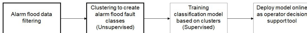
Figure 4.1: Pipeline of alarm flood diagnostic tool implementation. The bolded squares correspond to what was completed during this workshop.
