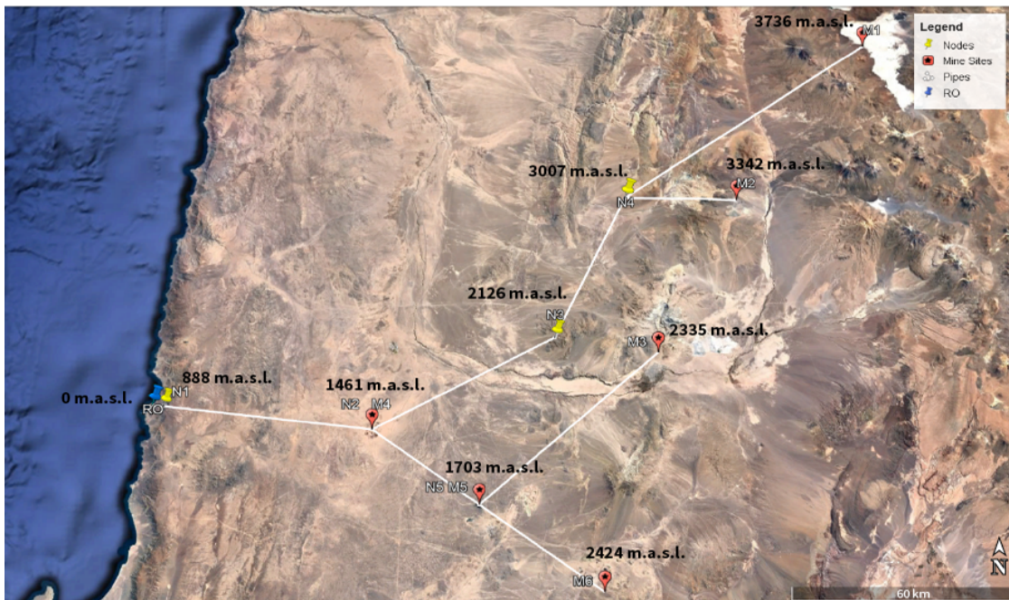
Figure 2: WSS proposed by Herrera-León et al. (2018a) to supply six mining sites. Image made using Google Earth.
