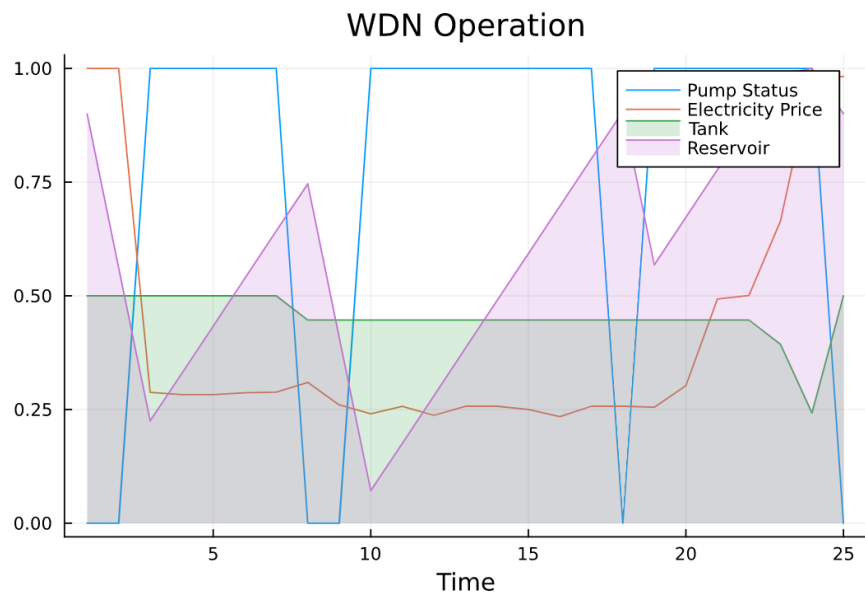
Figure 6: Example of a WSS with one pump and its expected results for the Water Pump Scheduling Problem. The volume of the water tanks and reservoirs, the electricity price, and the water pump status values are normalised and displayed in the same plot to analyse its variation per hour.
